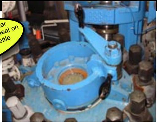
Opened DN 300 fill in cap on manhole cap with winder clasp and PEREL® handhole-seal.
